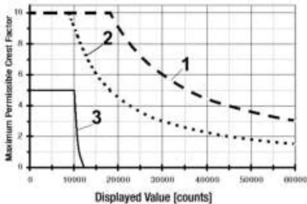
Additional error caused by signal's crest factor:  $1 < CF < 3$ : 1% R + 30D
