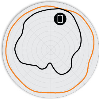
Figure 2. R650 2.4GHz Azimuth Antenna Patterns
