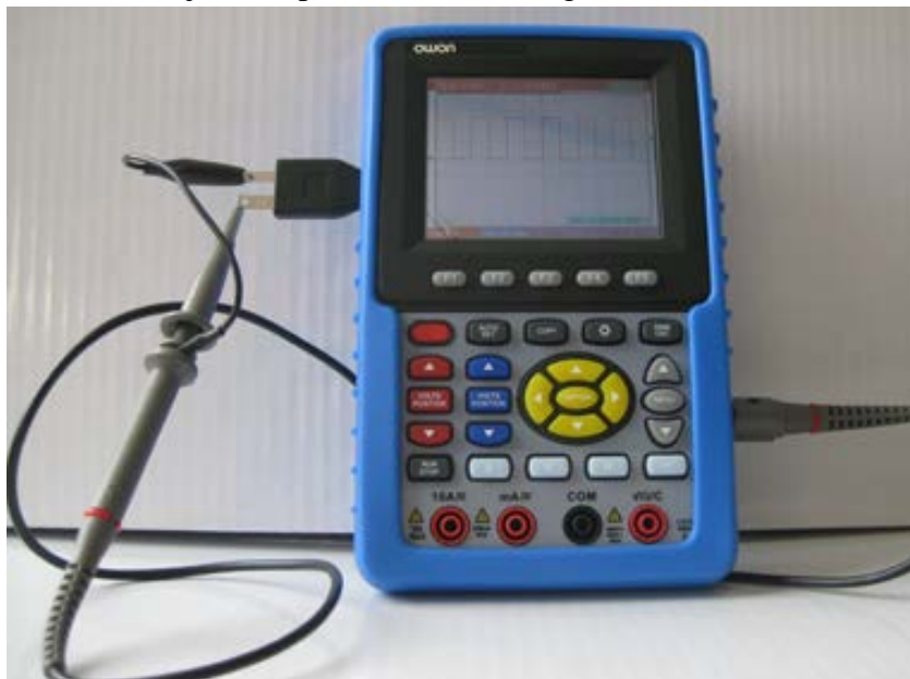
Fig.3. The connection of Square-wave test signal
