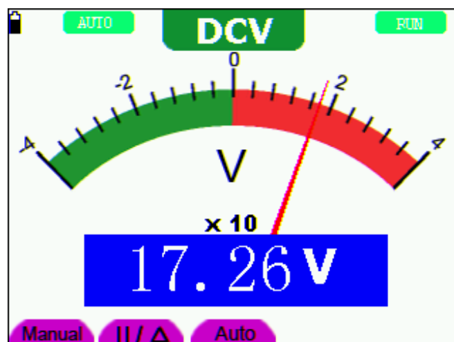
Figure 25: DC Voltage Measurement
