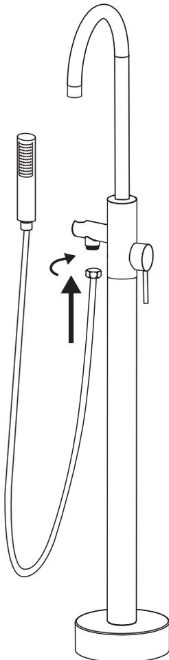
6. Install the hose to the handshower and the tub filler. Please check the tub filler spout and handshower water flow and its function.
