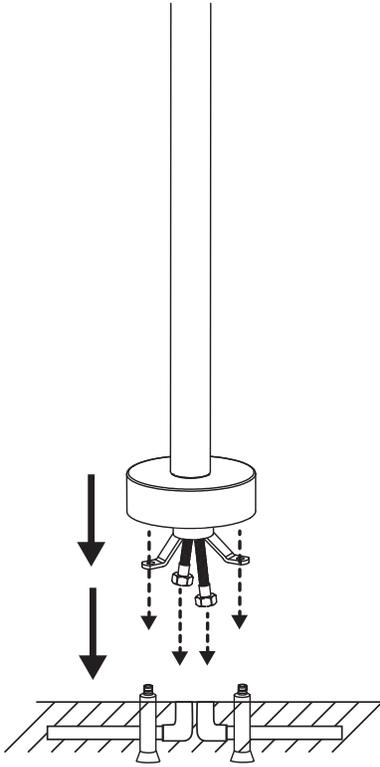
5. Tighten the screws to the floor mount on the ground. Insert the flexible hoses to the hot and cold outlet tube.
