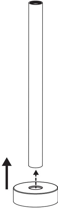
1. The floor escutcheon through the straight tube from top to bottom.
