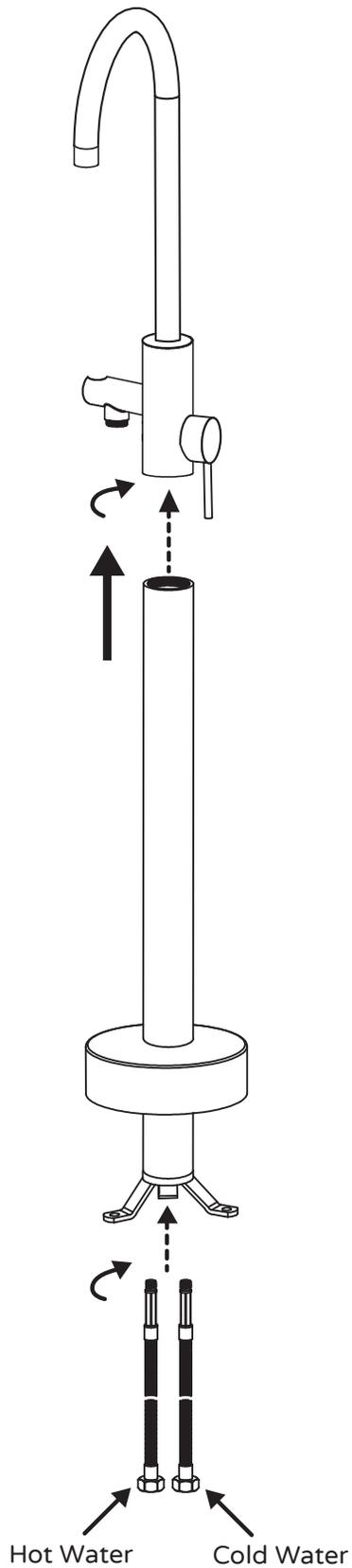
3. The flexible hoses through the straight tube. Twist tight to attach flexible hoses to faucet.
